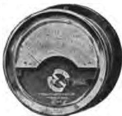
FIG. 64.—Hot-Wire Ammeter or Current Measurer.
